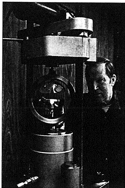
Lab manager Al Miller calibrates a "proving ring standard" in the Combatant Craft Department's testing facility at Fort Monroe, Virginia. CCD conducts extensive instrumented trials on hulls and marine systems to quantify performance characteristics.
