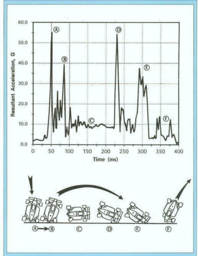
THE DATA HAS BEEN SLIGHTLY REVISED TO maintain the confidentiality of the driver and team, but the resultant plots are typical of a high-speed IndyCar crash into a solid barrier. The driver sustained no injuries. The analysis is based on a video film of the general vehicle path, and crash dynamics data from the onboard impact recorder.
