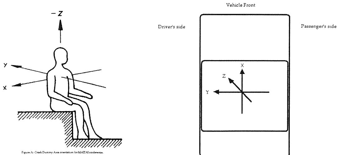
Figure A: Crash dummy axis orientation
